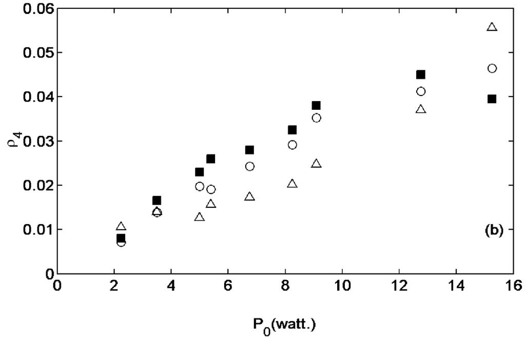
Figure B.8: Comparison between the experimental measurements (filled squares), simulations without stochastic phase fluctuations (open triangles) and with stochastic phase fluctuations (open circles) of the first-order sideband power versus pump input power for  $L=50.39$  m, and  $\Omega = 366$  GHz: power in the (a) blue-shifted sideband and (b) red-shifted sideband.
