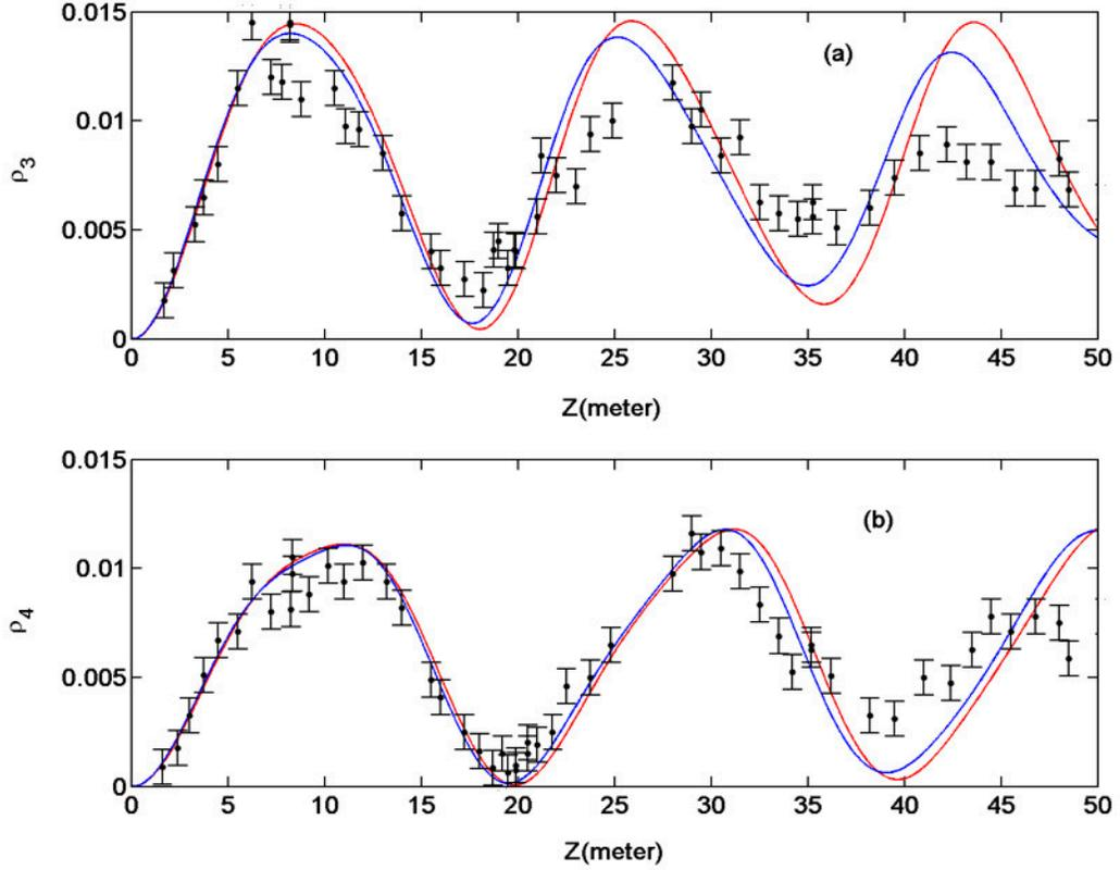
Figure A.4: Effects of inclusion of the pulsed nature (5 ns FWHM) of the input pump laser light on the first-order sideband evolution as a function of fiber length for  $P_0 = 2.1$  W. Dashed curves represent cw simulations and solid curves represent pulsed simulations.  $\Omega = 366$  GHz,  $\Delta\nu = 0.5$ ,  $\gamma = 0.019$  W $^{-1}$ m $^{-1}$ , and  $\beta^{(2)} = 55$  ps $^2$ /km (a) power in the blue-shifted sideband, (b) power in the red-shifted sideband.
