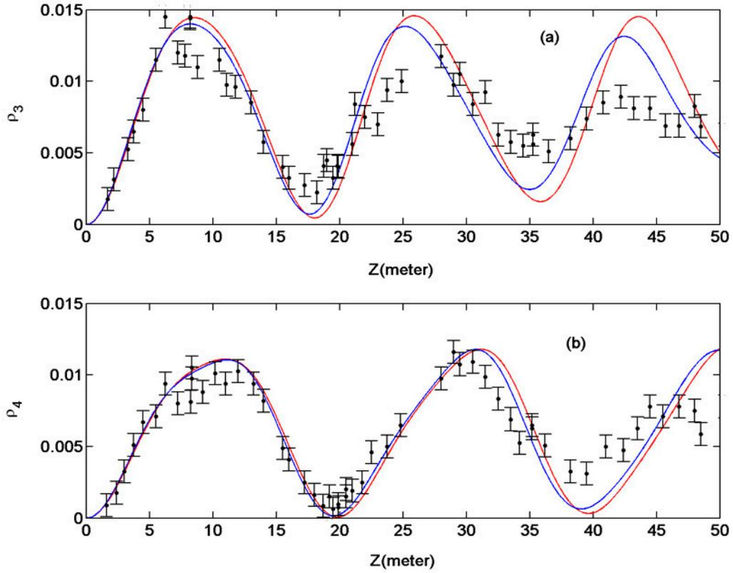
Figure 3.4: Effects of inclusion of the pulsed nature (5 ns FWHM) of the input pump laser light on the first-order sideband evolution as a function of fiber length for  $P_0 = 2.1$  W. Dashed curves represent cw simulations and solid curves represent pulsed simulations.  $\Omega = 366$  GHz,  $\Delta\nu = 0.5$ ,  $\gamma = 0.019$  W<sup>-1</sup>m<sup>-1</sup>, and  $\beta^{(2)} = 55$  ps<sup>2</sup>/km (a) power in the blue-shifted sideband, (b) power in the red-shifted sideband.
