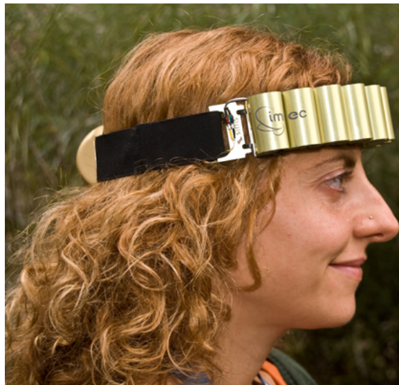
Figure 4.3: Example of the first available wireless EEG tool, made by IMEC. There should be a citation to the URL this photo came from.
