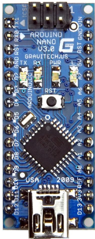
Figure 1.1: This is Arduino Nano
