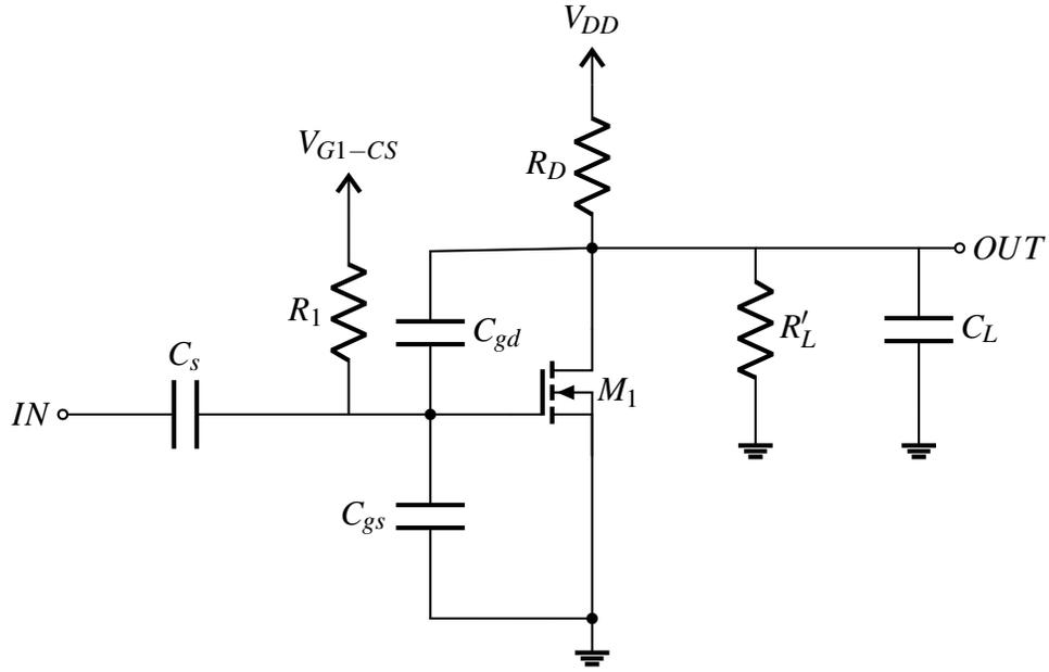
Figure 3.2: Common-source power amplifier circuit at high frequency.
