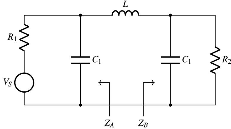
Figure 3.5: Typical circuit used for analyzing a  $\Pi$ -match network.
