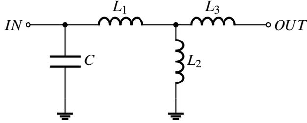
Figure 3.4: Input matching network of proposed CMOS power amplifier.
