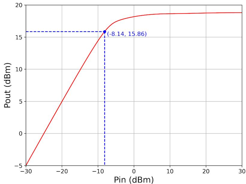
Figure 4.1: P1db compression curve of a single-stage power amplifier (shown in Figure 3.2).
