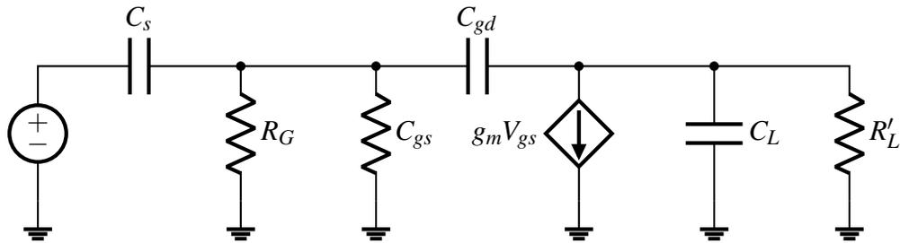
Figure 3.3: The CS power amplifier, a high frequency equivalent circuit shown in Figure 3.2.
