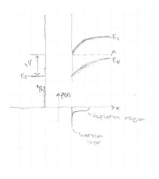
The pictures illustrated here explain a normally off (non conducting in the equilibrium state) NMOS (n-channel conducting) device on p-doped substrate. We also discussed how to adapt this model to oppositely doped devices and metals that had equilibrium fermi energies that were specially chosen to cause enough band bending to induce an inversion layer without the presence of an applied voltage and create a normally on device.
