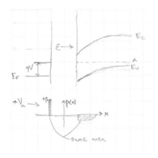
If the applied voltage meets a certain threshold, then the bands might bend so that the band furthest from the chemical potential in the equilibrium state is narrowly separated from the chemical potential at the oxide interface. This creates a highly doped region called the inversion layer. The inversion layer allows for heavy majority carrier concentrations to develop at the semiconductor surface and creates a conduction channel between the two doped wells:
