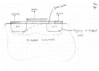
The reason we discussed the doped wells is because we wanted to show that the creation of a region doped in a similar way at the interface between the semiconductor and oxide would allow the two different wells to conduct between one another.
