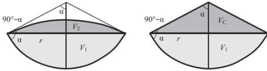
FIG. 1: Mathematical visual of the top of the droplet and peak. On the left is the top of the spherical, unfrozen water droplet.  $V_2$  is the volume of water taken from the drop before it froze. On the right is the peak of the frozen droplet. Notice the vertex angle,  $\alpha$  that the density ratio  $\rho$  depends on.
