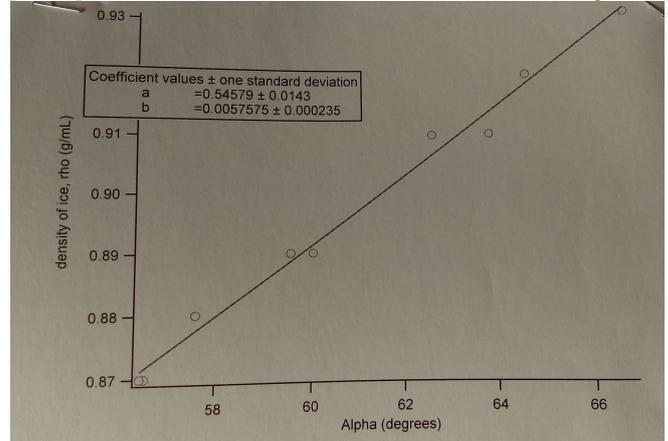
FIG. 3: The graph of the density  $\rho$  and vertex angle,  $\alpha$ . Ideally, the slope of this graph would be zero, since there is no mathematical dependence of the density on angle. However, due to slight variations in droplets, the slope of this graph is part of the calculation to find the uncertainty in  $\rho$ .
